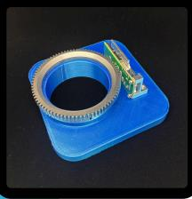
Hollow multi-turn absolute position encoder for robots
